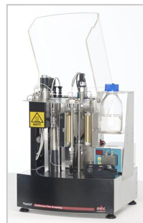
*HEL's new FlowCAT is a flexible and cost-effective choice in lab-scale Fixed-Bed Hydrogenation*
