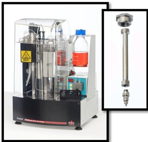
Experiments were performed in a standard ¼” internal diameter flowCAT reactor with automatic control of substrate flowrate, hydrogen feedrate and working pressure & Temperature.
