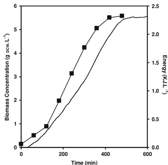
**Fig. 3** Comparison of biomass growth kinetics from a typical parallel *E. coli* TOP10 pQR239 fermentation based on off-line OD<sub>600</sub> measurements and the integrated heat generation curves: (■) OD<sub>600</sub>; (–) integrated heat curve
