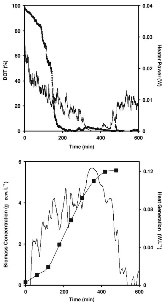
**Fig. 2** On-line heat measurements during a typical *E. coli* TOP10 pQR239 fermentation. (a) Profiles of dissolved oxygen tension and power supplied by the heater to maintain the fermentation at 37°C: (○) DOT; (–) heater power. (b) Comparison of biomass growth kinetics from off-line OD<sub>600</sub> measurements and calculated heat generation: (■) OD<sub>600</sub>; (–) heat generation
