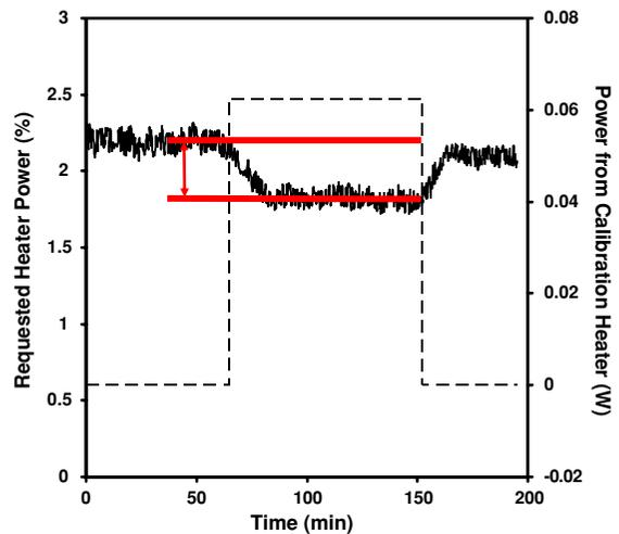
**Fig. 1** Calibration of the requested power of the electrical heater (—) used for temperature control of the miniature bioreactor. A known power was introduced to the vessel using a calibration heater (---). The average decrease in requested power when the calibration heater was activated, as indicated by the arrow, was 0.4%. Calibration was performed using a well-lagged vessel containing fermentation medium
